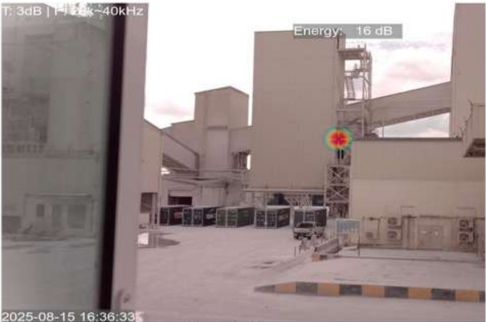
Detect leaks from 85m away. Sound energy 16dB
